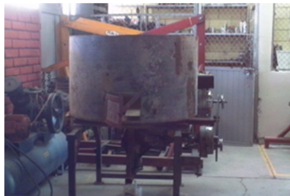
b. Large, stationary electric mixer with a differential from a car engine (#2)
