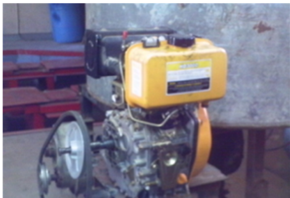
a. Motor and tank of large capacity stationary diesel mixer that can run on biodiesel (#1)
