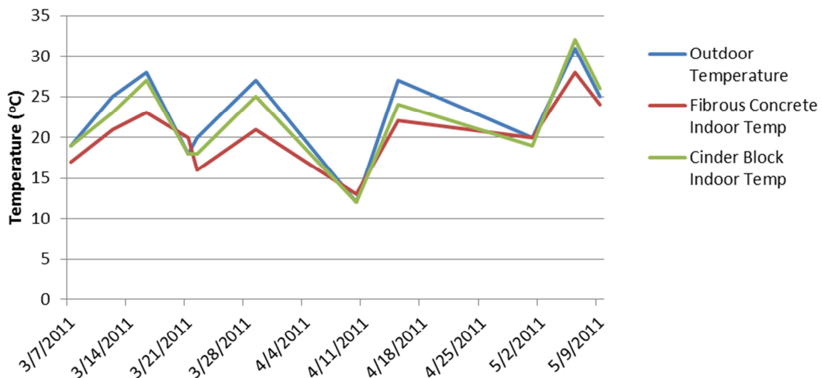
Figure 3.3. Afternoon temperature variation in homes with fibrous concrete and cinder block walls
