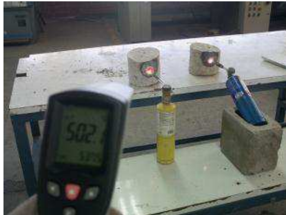
Figure 2.5. Test for Fire Resistance
