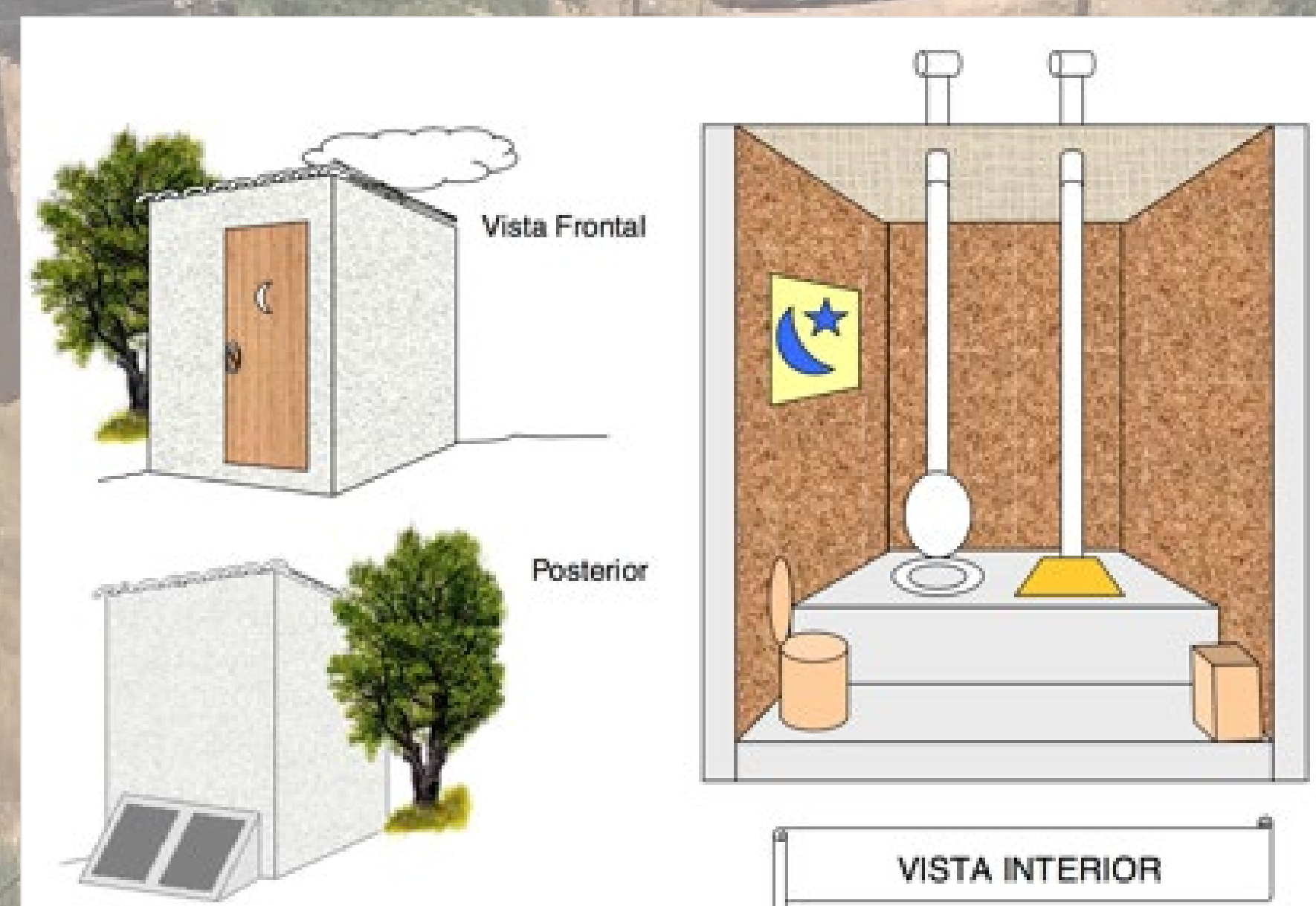
Diagram of a double-chamber composting toilet, the model used in Colinas del Sol
